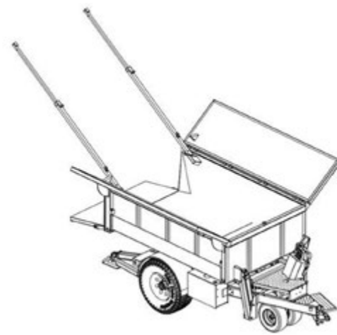
Figure 27. Rear Extension Rails Installed
